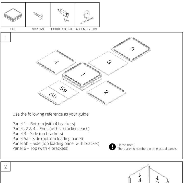
One at a time, place panels 2, 3, and 4 into the brackets on panel 1 and the adjoining corner brackets, ensuring that panels are square and fully inserted into the brackets.
